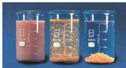
The principle of flocculation with our high grade fission powder **aquafloc\*7**
