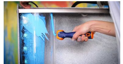
Cleaning the rollers with 3 - 4 bar water pressure ( rotoclean*N )
